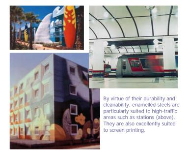
The steel industry has developed enamelling steels, including one with an aluminium-silicon coating that promotes adhesion of the enamel.
